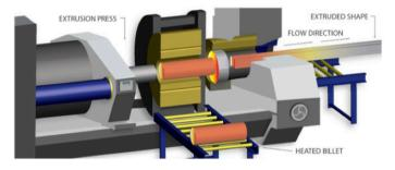
Figure 2. A rendering of the aluminium extrusion press die exit. Source: AMETEK Land
