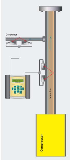
FLUXUS® G601 CA Energy is not only capable of measuring the flow rate of liquids, but also thermal energy quantities and flow rates of industrial gases. Thus, the FLUXUS® G601 CA Energy has especially been designed for the non-intrusive flow measurement of compressed air.
