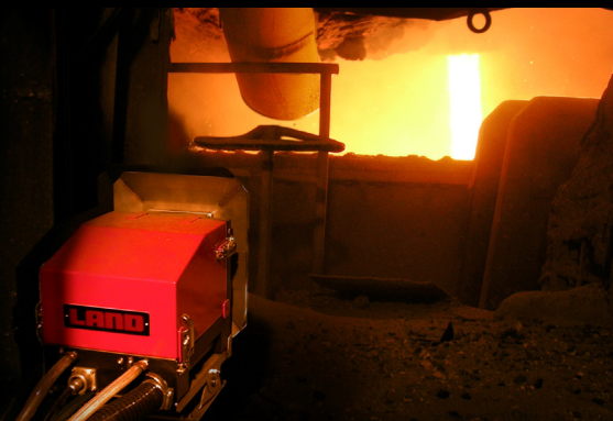
The Slag Detection System has a robust housing assembly, which views directly the liquid metal stream as the steel is tapped.
