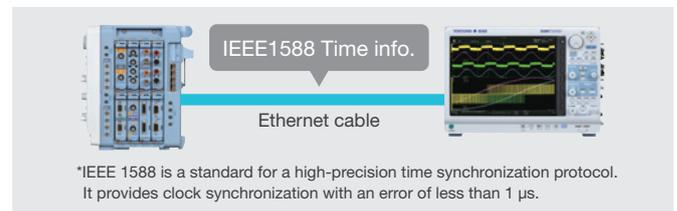
\*IEEE 1588 is a standard for a high-precision time synchronization protocol. It provides clock synchronization with an error of less than 1  $\mu$ s.
