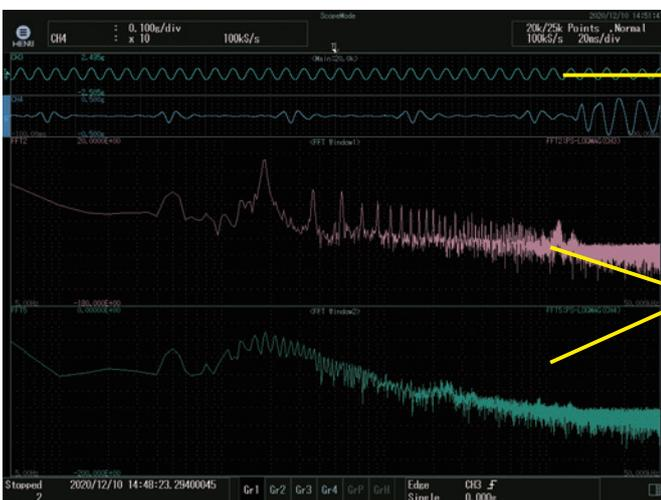
Vibration detection with acceleration pickup
